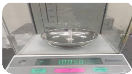
Figure 3. Eppendorf Tube Weighed 3 Times on a Precisa Electric
