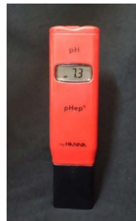
Figure 3. Digital pH Meter Used for Analyzing Salivary pH
