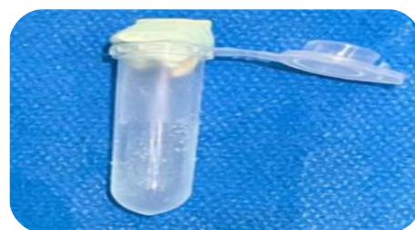
Figure 1. Teeth Mounted on Eppendorf Tubes Using Putty
