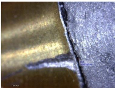
**Figure 1.** Image of the Frame Before Porcelain Firing Procedure Obtained With a Stereomicroscope at 204×Magnification
