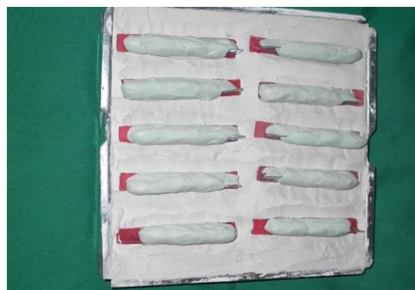
Figure 2. Investment of The Specimens With Silicon
