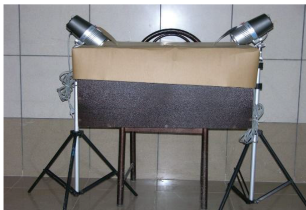
Figure 3. Dark Box, Placement of The Camera Lens and of The Light Source
